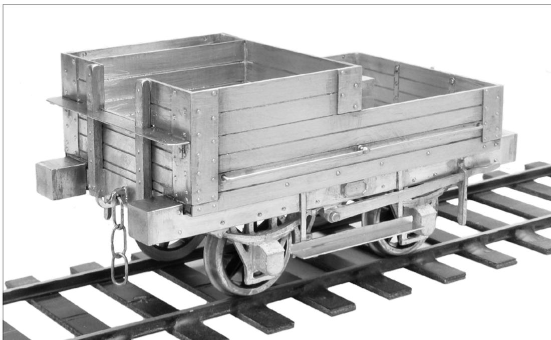
**Prototype.** Tender trucks of this type were coupled to small tank locos to provide extra coal supplies and carry the tools and equipment required for a long days work in sidings remote from the main loco depot. They were fitted with footboards and handrails to allow staff to ride along safely between shunting movements
