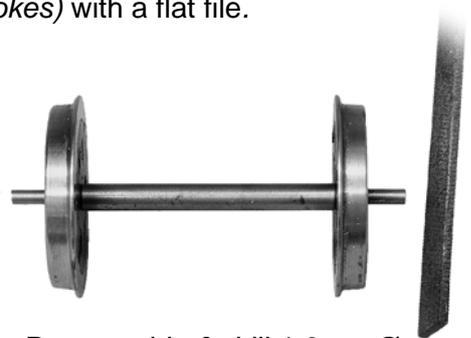
Reassemble & drill 1.6mm Ø hole down & through stretcher, aligning all holes.
