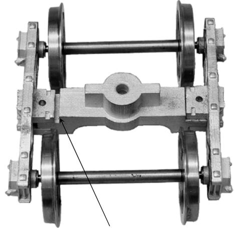
Note gap on stretcher when using Slater's wheelsets. My preferred solution is to reduce axle width by filing off the pin points (plus a couple of strokes) with a flat file.
