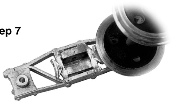
Offer up wheelset to check clearance. Make adjustments as required (*possibly chamfer brake block rear with knife blade*). When happy solder solid & clean up. Ensure rebate for stretcher end is clean & clear.
