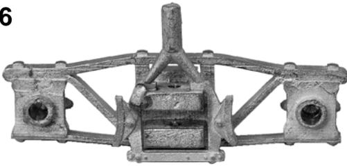
When happy with basic bogie, disassemble & fit brake yoke using a single tack solder joint.
