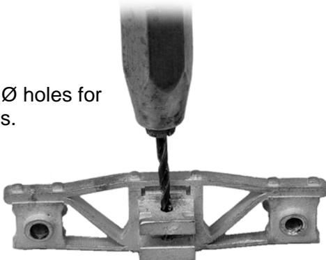
Drill & break through from top and then bottom. Then gently run drill right through to align both holes.
