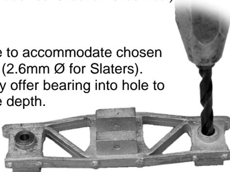
Hold drill in hand pin chuck for maximum control to help prevent breaking through axlebox front.
