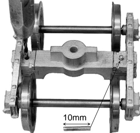
Cut from brass rod & fit assembly pins .
