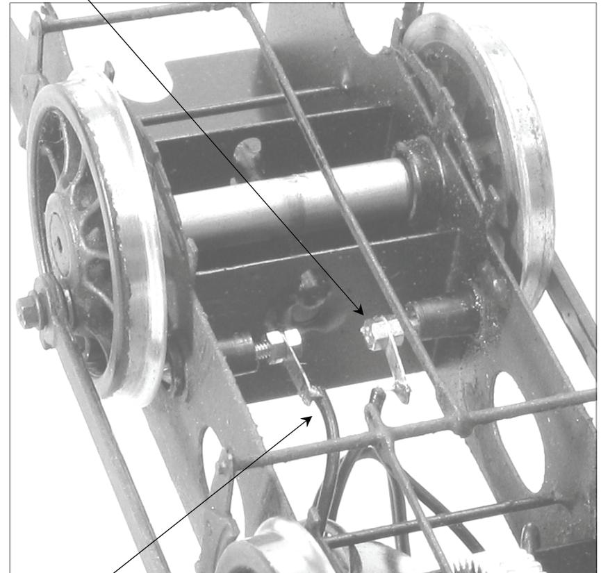
Also note how the electrical wire is gently curved so as to allow movement of the pickup
