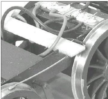
Wire wiper pickup system consisting of PCB strip glued across the chassis. Wiper wire made from 0.45mm brass wire (note how end is formed into loop to provide a good contact area on the wheel tread) and insulated electrical wire to take electrical power to the motor.
