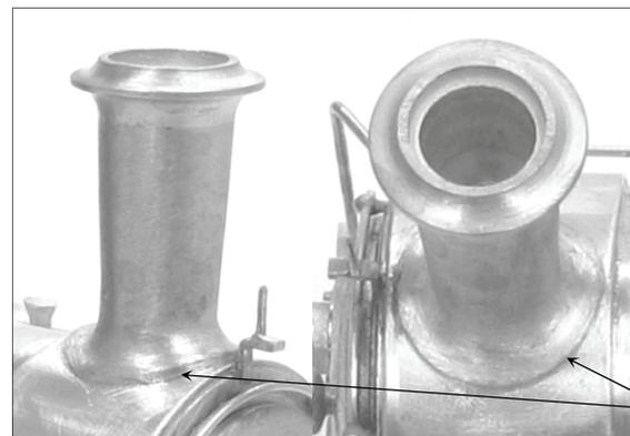
The chimney has been soldered into place with a generous fillet of 70° solder run around the base. Then using a curved scalpel blade the excess solder has been scraped back from the brass smokebox and a fibreglass brush worked around the base of the flange to reveal a distinctive circular edge to the casting and feathering the solder into the brass.
