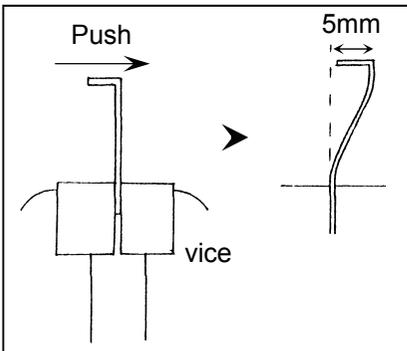
Clamp the top part of the cow catcher in the jaws of a vice and push the angle iron forwards until the bottom becomes offset from the top by 5mm. Ensure that the angle iron remains parallel to the jaws of the vice.
