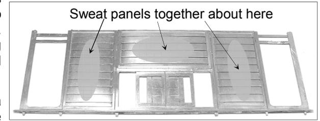
You will probably find that a little solder has got onto the surface of the parts and that they have discoloured a red/pink colour due to the heat. This should be easily corrected by burnishing with a glass fibre brush.
