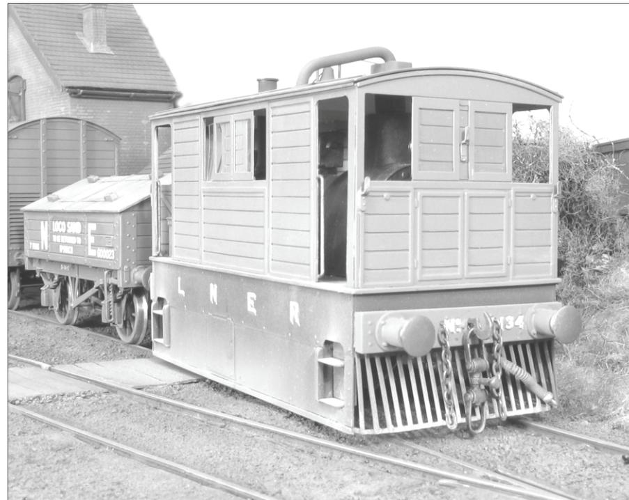
The first members of this class of 10 engines were built in 1883 for the opening of the Wisbech & Upwell tramway and the last two members of the class were completed in 1897. They were designed to meet the rigid specification laid down by the government for railway locomotives operating along public roads. These included full side skirting and enclosed bodywork to prevent frightening the horses and the ability to drive from each end so as to achieve the fullest view of the road ahead.
