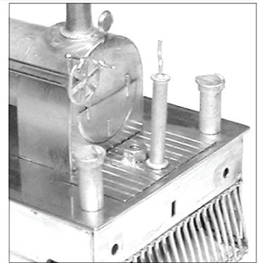
There are now two options for the main body. You can fix it in place on the footplate by soldering around the bottom edge ensuring that the footplate projects an equal distance from the sides and ends. As the boiler can be left removable until after painting you should not have any difficulty brush painting the interior.
