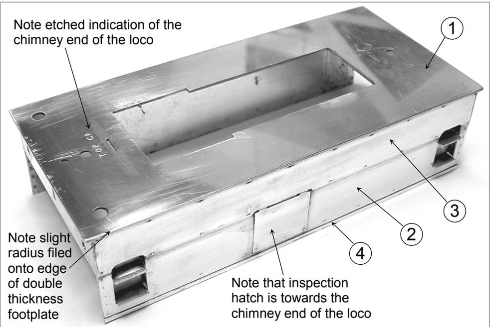
Note slight radius filed onto edge of double thickness footplate
