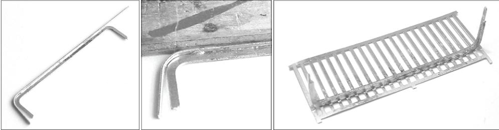
Pin the cow catcher bars (parts 27) to a flat surface and solder the angle iron to the bars at the point where the bars become half etched. Do not solder the two outer bars on either side as these are to be fiddled round the corners later. Then trim off the excess length flush with the bottom of the angle iron.
