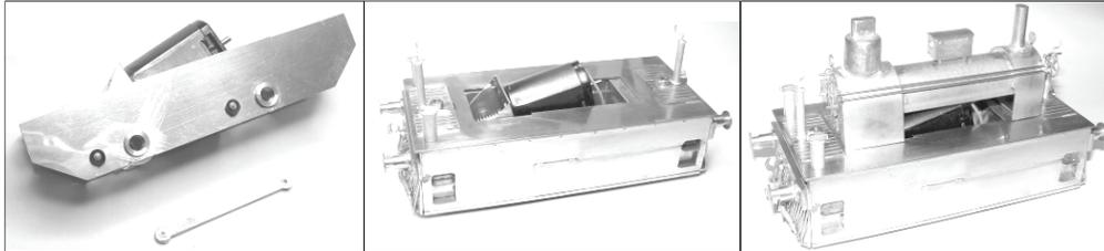
When happy, tack solder the mounting plate to the sideframes and remove the motor and bearings. You will note that the reason for the two oval slots in the spacer is to allow screwdriver access to the motor fixing screws.
