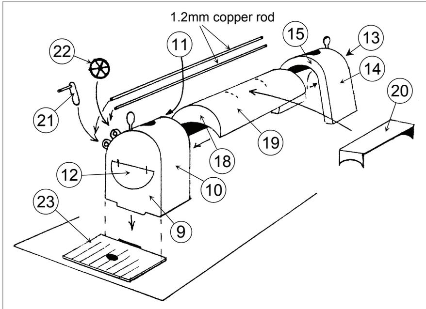
I would recommend first roughly pre forming the boiler, smokebox and firebox wrappers. As these are half etched they are easy to work around lengths of tube or dowel using finger and thumb pressure. Once they are roughly curved the end components can be used as formers to fix the final radius.
