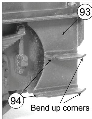
Fold a set in each guard iron (parts 95) using the etched marks as guides. Solder into the slots on the underside of the footplate. Tweak the folds on the guard irons with long nosed pliers to achieve a distance of 32mm (track gauge) apart and reinforce the fold lines with solder.
