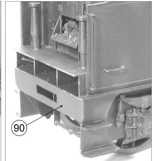
6. Fold the tender back steps (parts 89) through 90° and solder into half etched rebates. Fit the front drag beam (part 90) locating into the half etched groove on the underside of the footplate. Emboss bolt heads on the tender frames (parts 91) and fit into slots on footplate underside so that the end is hard against the front buffer beam. Fit the rear buffer beam (part 92) tight up against the ends of the frames.
