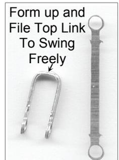
that they will pivot freely in the slot in the hooks. Thread one of these links through the hook and spring the ends over the pegs on the cast centre. Then fit the bottom link. Pass the coupling hook through the slot in the buffer beam, I solder it solidly into place but you can retain it with a spring if you wish.
