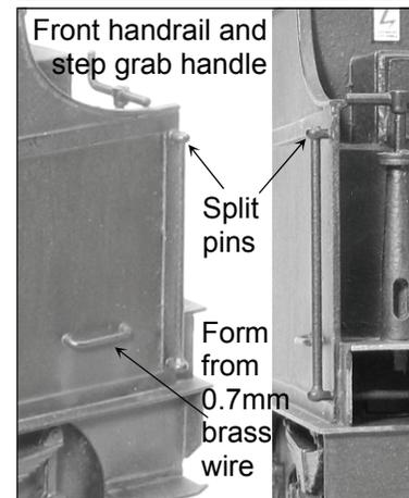
The handrails are formed from 0.7mm brass wire. Only the front handrails were supported by any form of handrail knob and even if you normally use handrail knobs I would recommend using the split pins as they better represent the prototype supports.
