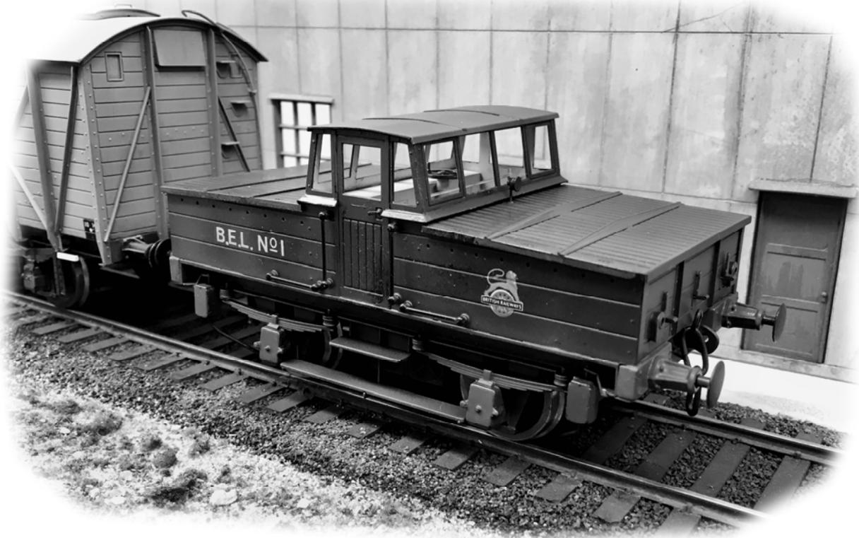
This is an etched brass construction kit based on the battery electric locomotive that worked the Midland's coal depot near West India Dock in Poplar, East London from 1913 to 1964. There was no rail access to the depot the only means of access was by a hydraulic wagon hoist hence the size, height and weight of the loco which had to use the hoist for maintenance or overhauls. A number of similar locos were produced to suite industrial locations.
